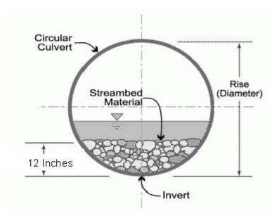
In all other counties: Culverts greater than 48 inches in diameter will be buried at least one foot below the bed of the stream. Culverts 48 inches in diameter or less shall be buried or placed on the stream bed as practicable and appropriate to maintain aquatic passage, and every effort shall be made to maintain the existing channel slope. The bottom of the culvert must be placed at a depth below the natural stream bottom to provide for passage during drought or low flow conditions.
